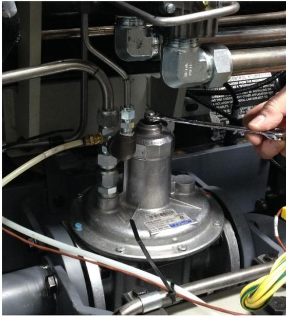
Figure 12-Regulator Adjustment Device
