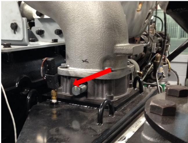
Figure 11-Carburetor Screw
